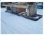
problem was mostly solved by building a giant flat bottomed sled which slides over the ice and does not sink in the mud, capable of carrying
